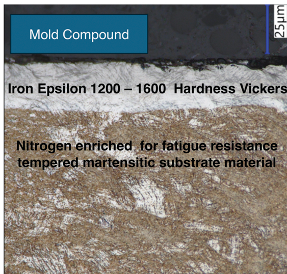
15-5 Martensitic Stainless Steel – 500 X
